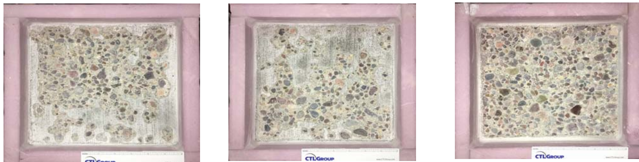
Figure 2. Control samples without waterproofing product and curing compound after 100 cycles of freezing and thawing
