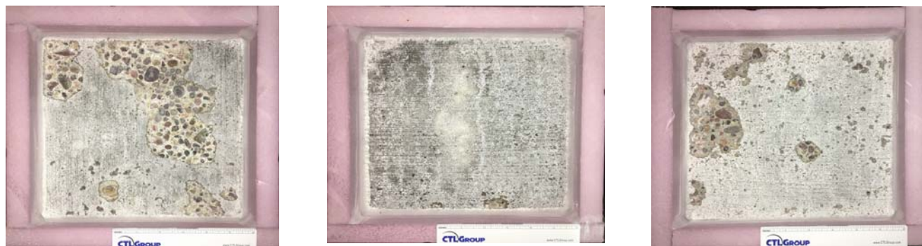
Figure 1. Samples with waterproofing product and curing compound after 100 cycles of freezing and thawing
