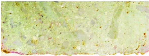
Figure 8: Absorption test for treated and untreated post samples
