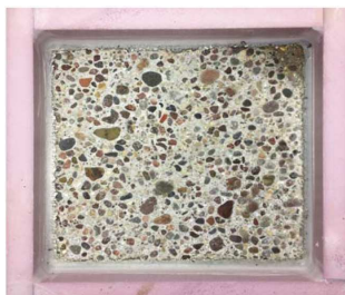
Control sample without Pavix and curing compound after 70 cycles of freezing and thawing
